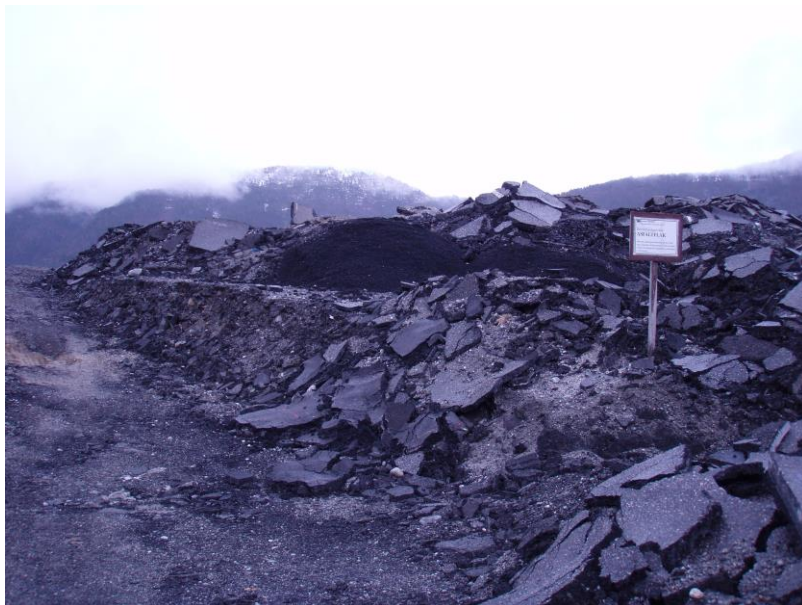
Storage-site for RAP (asphalt waste materials).
